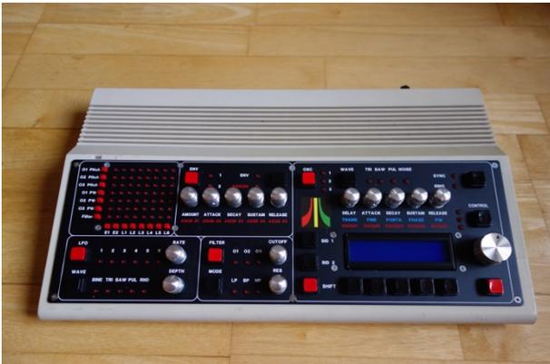
Figure 2 : MIDIbox SID synthesizer (Jahtari, 2014)
