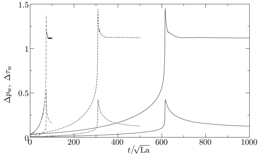
FIG. 10. The effects of the liquid viscosity on the time evolution of the excursion of wall stresses  $\Delta p_w$  (higher-amplitude curves) and  $\Delta \tau_w$  (lower-amplitude curves) for  $\varrho = 10^{-3}$ ,  $\lambda = 6$ ,  $\varepsilon = 0.25$  and  $\text{La} = 1$ ,  $\mu = 1.5 \times 10^{-4}$  (solid line),  $\text{La} = 4$ ,  $\mu = 3 \times 10^{-4}$  (dashed line),  $\text{La} = 100$ ,  $\mu = 1.5 \times 10^{-3}$  (dashed-dotted line).
