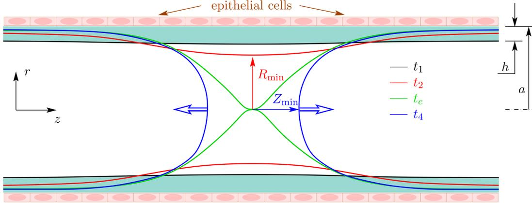
FIG. 1. Schematic of the airway closure process. The air–liquid interface is depicted at four instants of time: for  $t = t_1$  the interface is slightly deformed, for  $t = t_2$  the deformation has increased because of the Plateau–Rayleigh instability, for  $t = t_c$  it coalesces while undergoing a topological change, and for  $t = t_4$  the newly formed liquid plug undergoes a bi-frontal growth.
