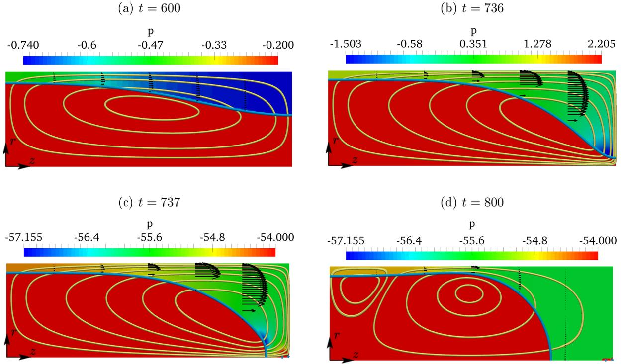
FIG. 6. Pressure field (colors), streamlines (yellow lines) and axial velocity in the liquid phase (arrows) at two pre-coalescence (a:  $t = 600$  and b:  $t = 736$ ) and two post-coalescence instants (c:  $t = 737$  and d:  $t = 800$ ). The turquoise line denotes the interface location. The phenomenon is symmetric in  $z$ .
