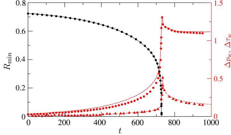
FIG. 14. Minimum of the interface radial location  $R_{\min} = \min(R_I)$ , excursions of wall pressure  $\Delta p_w = \max(p_w) - \min(p_w)$  and shear stress  $\Delta\tau_w = \max(\tau_w) - \min(\tau_w)$  computed with basilisk (lines) and with the numerical solver of Muradoglu et al. [55] (markers). The non-dimensional groups are  $La = 100$ ,  $\lambda = 6$ ,  $\varepsilon = 0.25$ .
