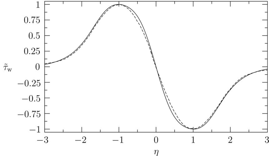
FIG. 13. Normalized wall shear stress  $\tilde{\tau}_w = \tau_w / \max(\tau_w)$  at  $t = t_s$  against the normalized coordinate  $\eta = z/z_{\tau_w, \max}$ . The present results (solid line) are compared to the results by Tai et al. [38] (dashed line).
