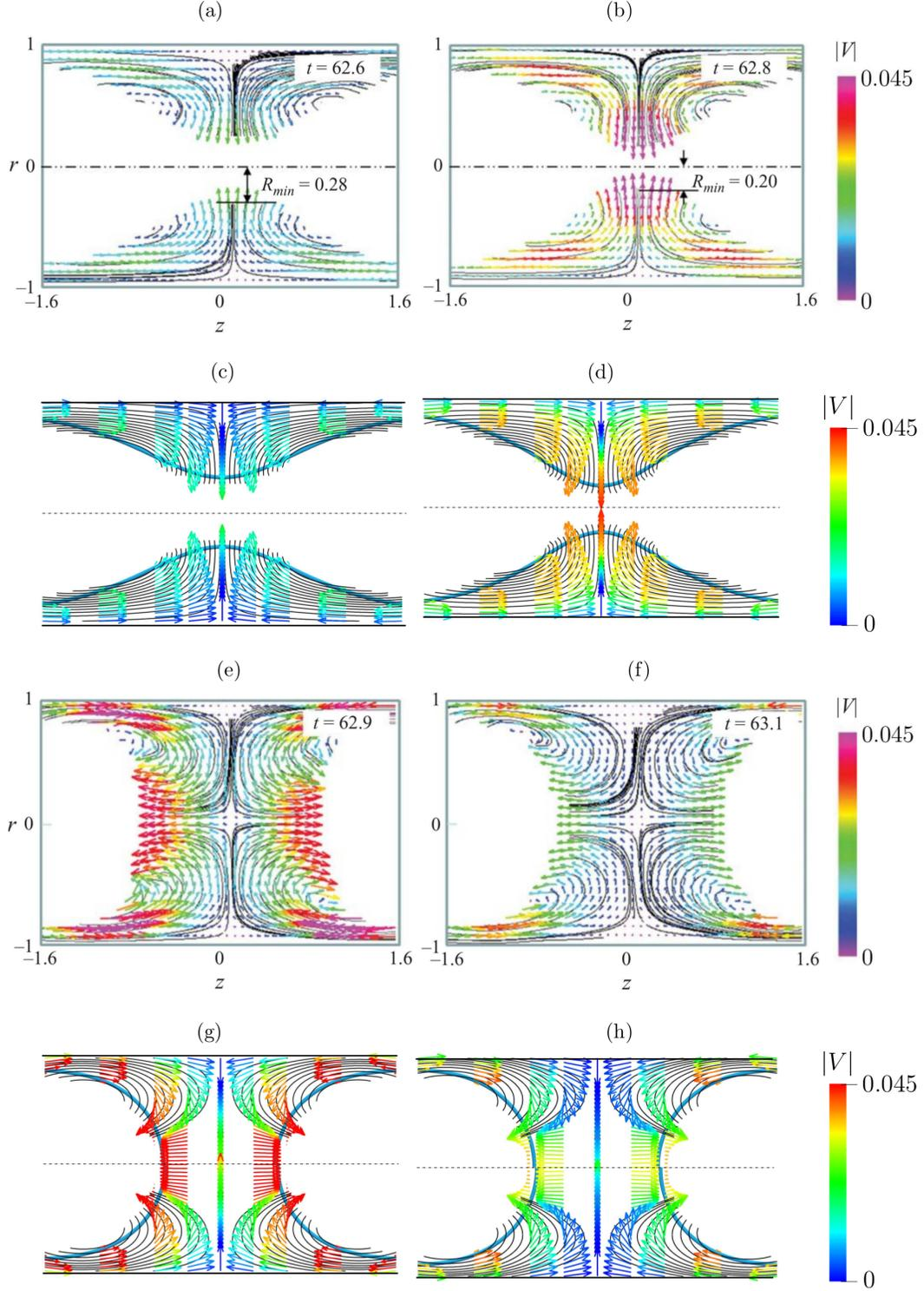
FIG. 4. Velocity vectors (arrows) and streamlines for  $\varepsilon = 0.23$ ,  $\text{La} = 0.072$ ,  $\mu = 0.01$ ,  $\varrho = 0.95$ ,  $\lambda = 9.2$ : first (a–b) and third (e–f) rows from the top are the micro-PIV measurements of Bian et al.[37], whereas second (c–d) and fourth (g–h) rows from the top are numerical results. Time is scaled by  $\mu_L a / \varepsilon^3 \sigma$ .
