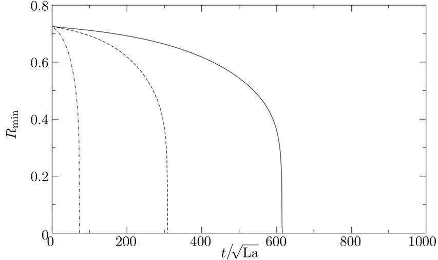
FIG. 9. The effects of the liquid viscosity. The time evolution of the minimum radius of the interface,  $R_I$ ,  $R_{\min}$ , is plotted for  $\varrho = 10^{-3}$ ,  $\lambda = 6$ ,  $\varepsilon = 0.25$  and  $\text{La} = 1$ ,  $\mu = 1.5 \times 10^{-4}$  (solid line),  $\text{La} = 4$ ,  $\mu = 3 \times 10^{-4}$  (dashed line),  $\text{La} = 100$ ,  $\mu = 1.5 \times 10^{-3}$  (dashed-dotted line).
