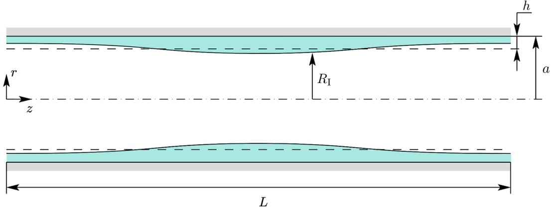
FIG. 2. Schematic of the geometry of the airway model: the rigid tube has radius  $a$ , length  $L$ , is coated by a liquid film (light blue) of average thickness  $h$  and surrounded by a gas core. The interface is initially located at a distance  $R_I$  from the axis of the pipe.
