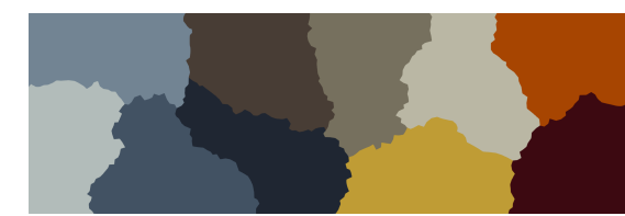
Figure 6: 2D mesh partition (10 processors)
