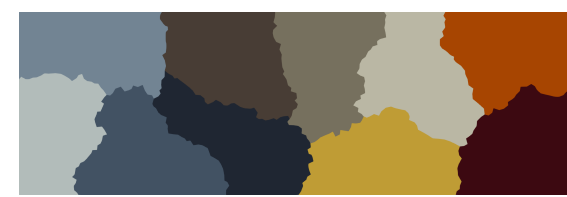
Figure 6: 2D mesh partition (10 processors)
