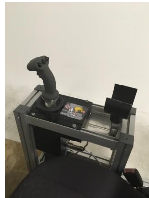
Figure 4: the ASSUs used respectively as collective stick (left) and cyclic stick (right)
