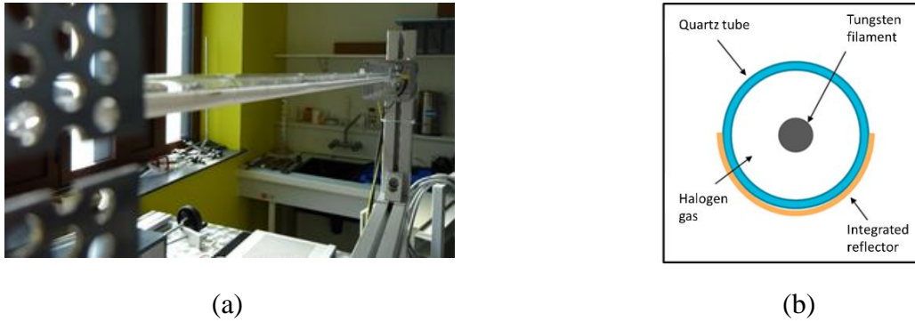
Fig. 1. (a) Infrared halogen lamp with integrated reflector, (b) Schematization
