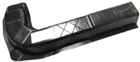
Fig. 2.: Thermoformed 3D final shape after QSP®
