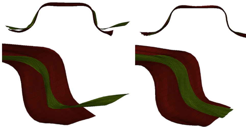
Fig. 14.: Interply behavior : without adhesion Fig. 15.: Interply behavior : with adhesion
