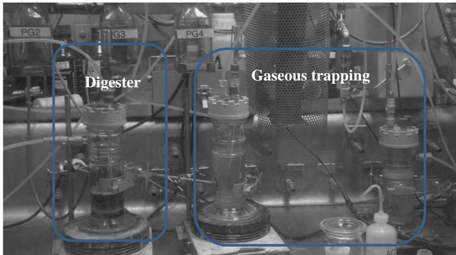
FIG. 1. Oxidative digestion setup.
