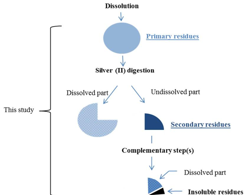
FIG. 2. Dissolution process flow diagram (simplified).
