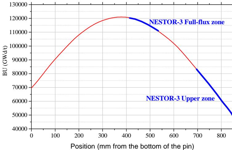
FIG. 4. Local burnup of NESTOR-3 dissolved pin parts
