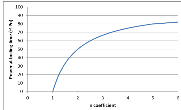
FIG. 3. Relation between the 'r' coefficient and the power at boiling time
