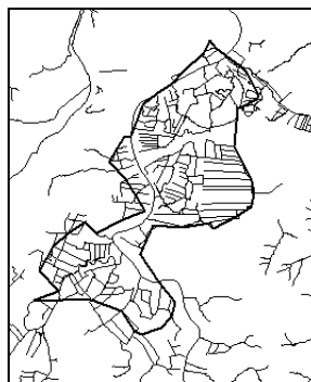
Fig. 8. Results of irrigation zone automatic creation : the bold polygon contours the irrigation area.
