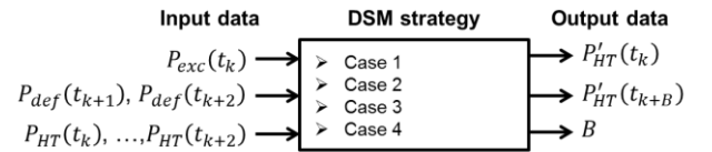
Fig. 5. Overview of the data related to the electric room heaters DSM strategy
