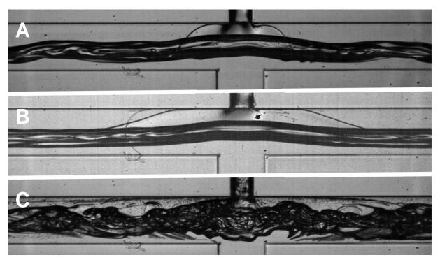
Figure 3.Image of the CCD camera in the impinging zone : Case A (top), B (middle) and C (bottom) - channel width : 600 µm.
