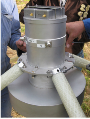
Figure 3. Photograph of a feed: The two amplifiers for the H and V probes are located in the two boxes at the top.
