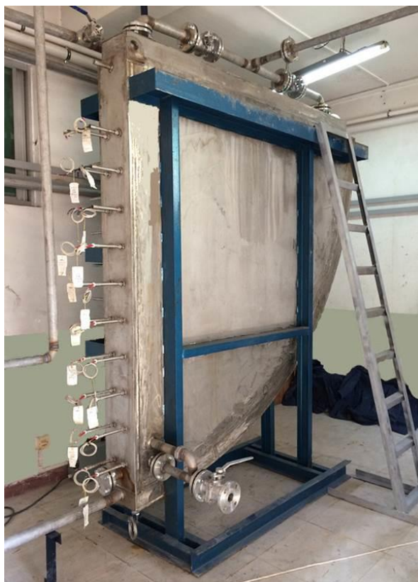
Figure 8. Test vessel of the COPRA facility
