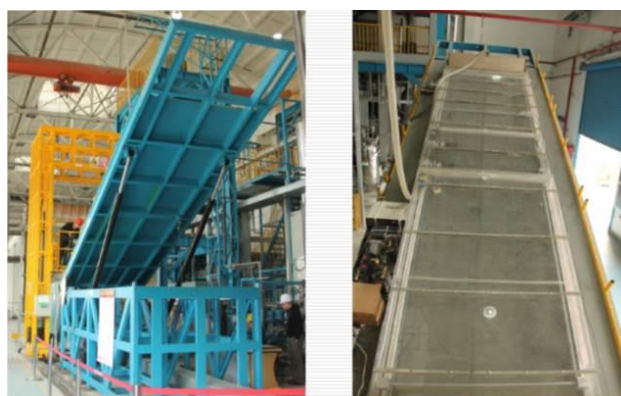
Figure 10. WAFT facility (left) and test section (right).
