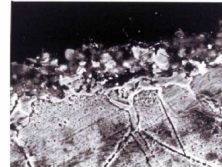
304 ds Na T = 550 °C – t = 60000h T = 600 °C – t = 20000h CREVONA loop (KIT) Ganesan et al., JNM 312 (2003) 174
