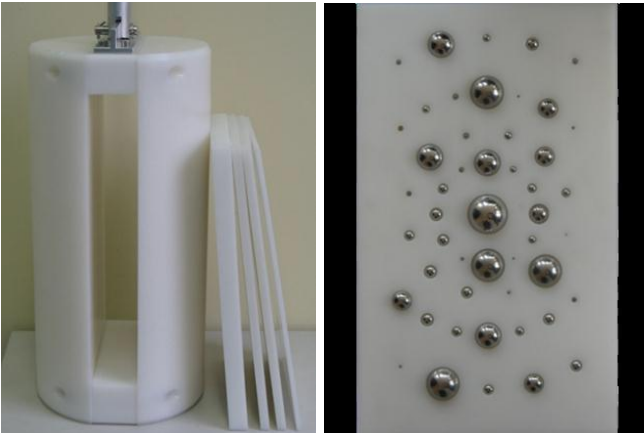
Fig. 3. Steel balls phantom: polyethylene cylinder (left). The inside of the cylinder is filled either with polyethylene or with the plate containing the balls (right).
