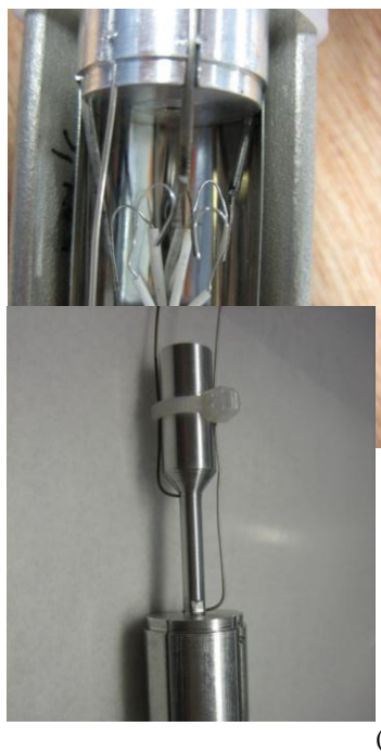
Fig. 3 – (a) 4-wires resistance implementation in lower cell, (b) New position of thermocouples on the pedestal
