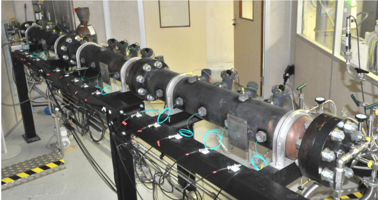
Figure 2. SSEXHY facility in the 3-modules configuration.
