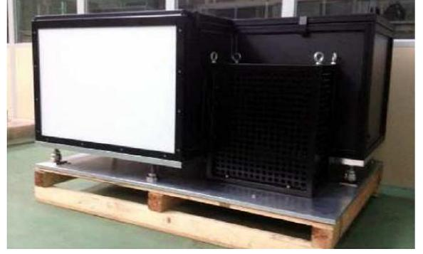
Fig. 5. 2D scintillator detector. The scintillator screen is imaged by a low noise camera through a 45° tilted mirror. The screen size is 80 x 60 cm<sup>2</sup>.
