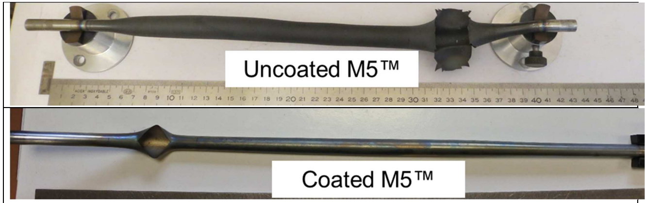
Fig. 4 Visual examinations of two tested clad segments after “EDGAR” creep tests performed at 600°C
