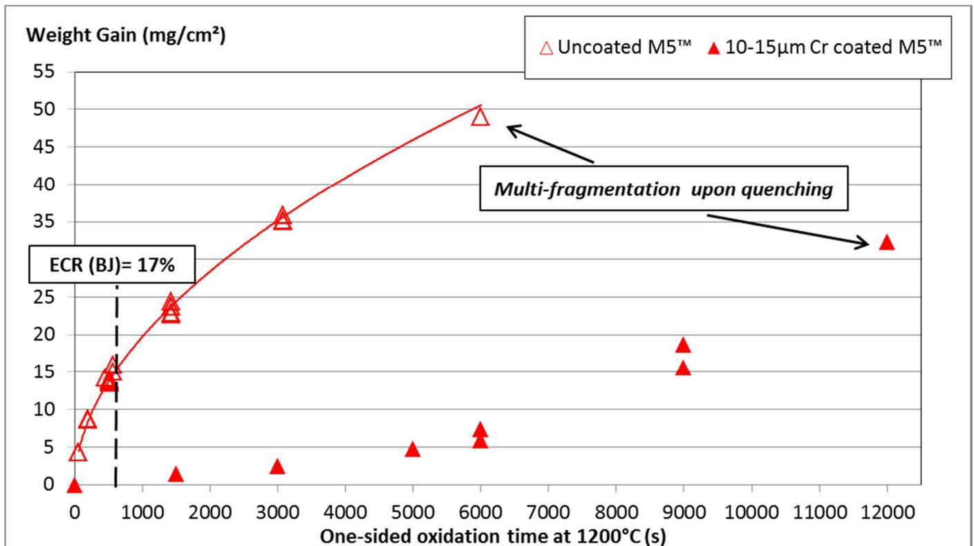
Fig. 6 Weight gain measured after one-sided steam oxidation at 1200°C and direct water quenching down to RT
