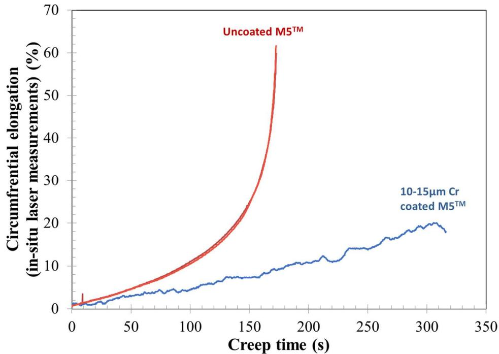
Fig. 2 Creep curves obtained on coated/uncoated M5<sup>TM</sup> claddings upon isothermal creep tests at 750°C, with the same applied internal pressure: two uncoated reference ones superposed, in red, and one standing for 10-15µm Cr coated (in blue)
