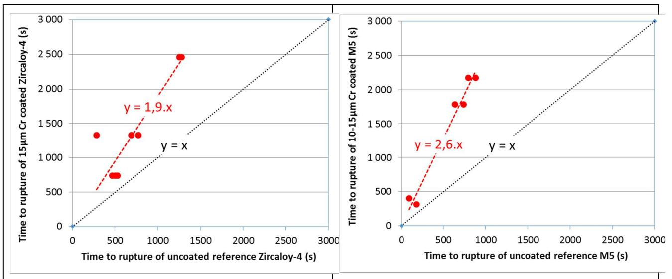
Fig. 3 Creep rupture times for Cr coated materials compared to those measured for uncoated reference ones (Zircaloy-4 – left and M5<sup>TM</sup> - right)
