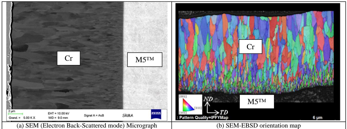
Fig. 1. Typical microstructure of a 10-15 $\mu\text{m}$  Cr thick chromium coating on a M5<sup>TM</sup> clad substrate
