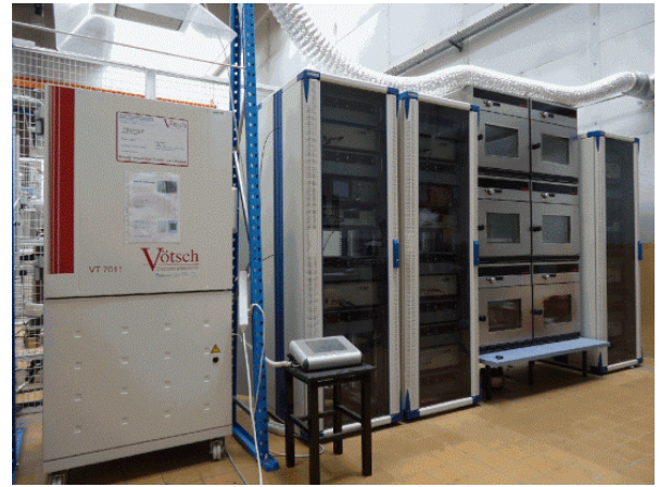
Fig. 2. The experimental setup for accelerated aging tests, climatic chambers and power electronic.
