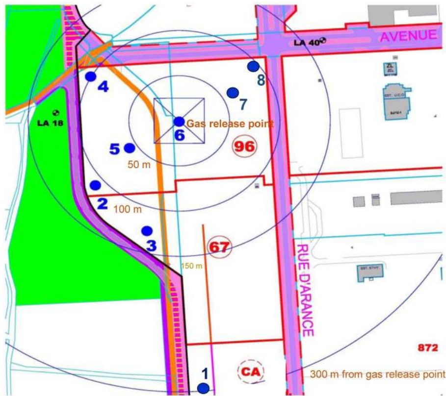
Figure 4—layout of the remote gas detection systems located at points 1, 2, 3, 4, 5, 7 or 8; the gas release point is located at point 6
