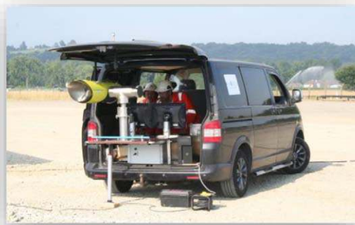
Figure 23—Gas Optics GVS® installed in a van
