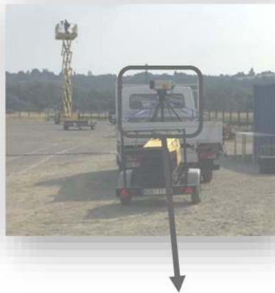
Figure 5—Telops Hyper-Cam installed on the bed of a pick-up
