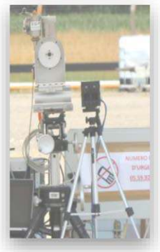
Figure 8—multispectral system with a cooled detector (left) and multispectral system with an uncooled detector (right)
