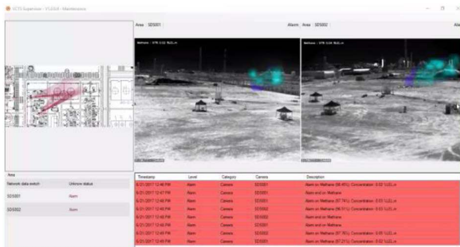
Figure 18—images of the Vapor Cloud Tracking System (VCTS) monitoring software
