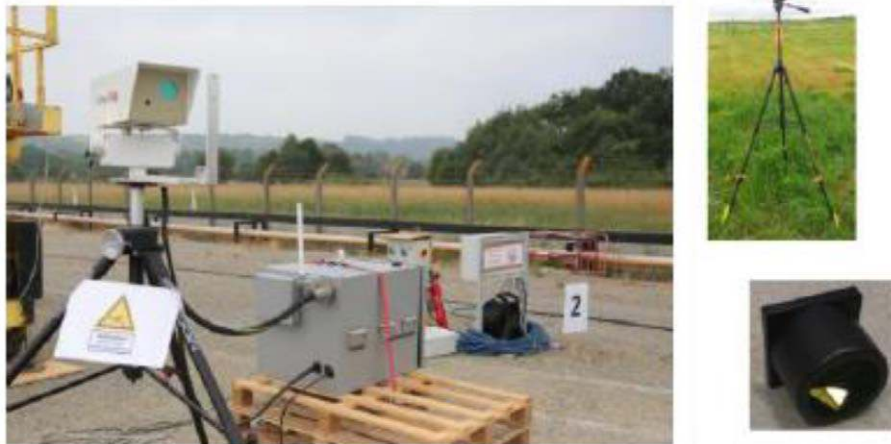
Figure 19—On left: Harris/AER GreenLITE™ Transceiver with Optical Head mounted on tripod and Electronics Box (2 per site) On right: Retroreflector mounted on tripod (30 per site)
