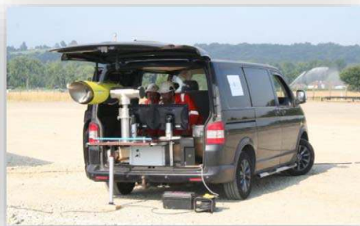
Figure 23—Gas Optics GVS® installed in a van
