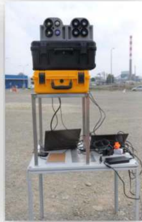
Figure 27—Fluke Gas Imaging Camera (GIC)
