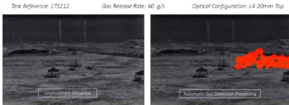
Figure 26—images obtained from the GSS during a gas release. The figures show the unprocessed image on the left and the image obtained when Automatic Gas Detection Processing is activated on the right
