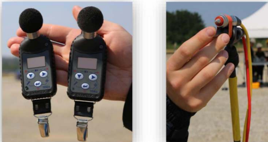
Figure 28—audible sonometers from SVANTEK on the left, ultrasonic microphone on the right
