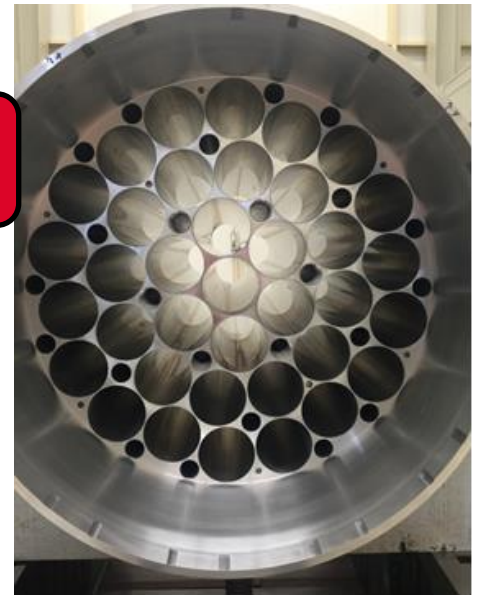
Rack for fuel elements
