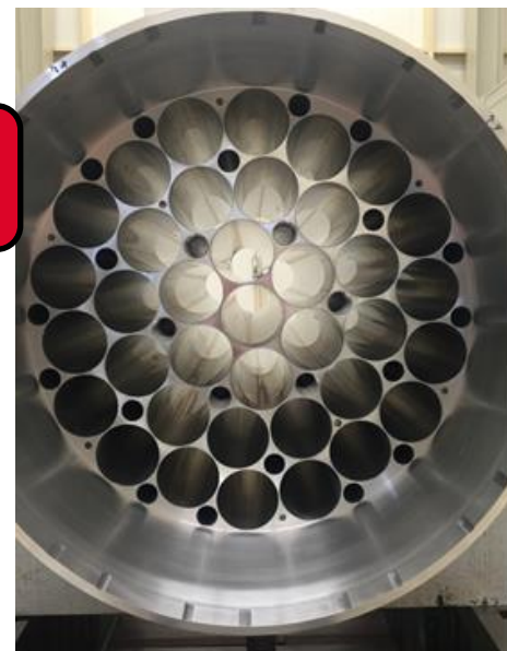
Rack for fuel elements
