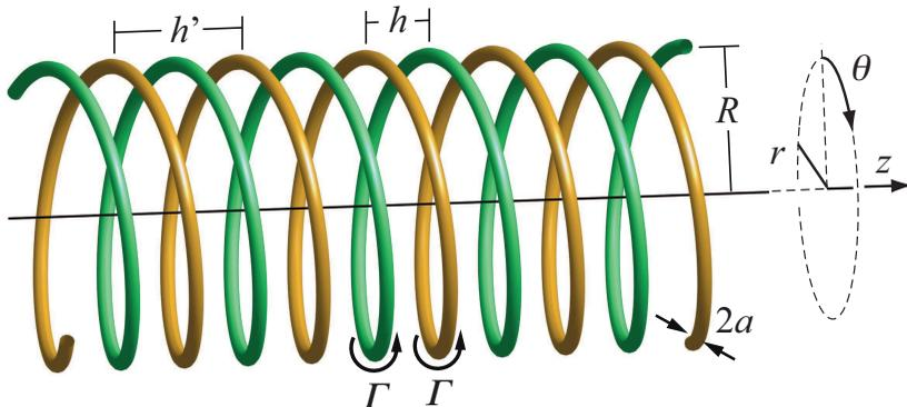
FIGURE 1. Schematic of two interlaced infinite helical vortices, including the relevant parameters: pitch  $h'$  of one helix, separation  $h$  of neighbouring helix loops, radius  $R$ , core size  $a$  and circulation  $\Gamma$ .
