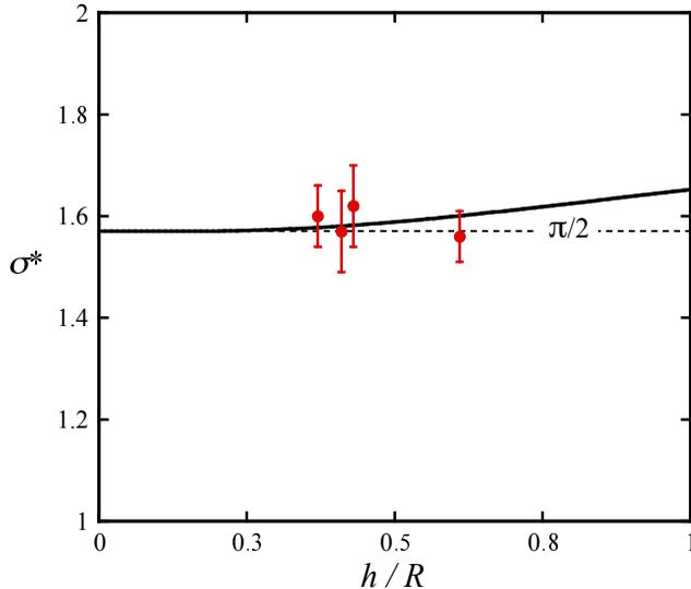
FIGURE 23. Growth rate of the long-wave instability due to global pairing, as function of the distance between neighbouring helix loops. Symbols correspond to experimental measurements, and the solid line is the theoretical prediction by Gupta & Loewy (1974) for  $a_e/R = 0.05$ .
