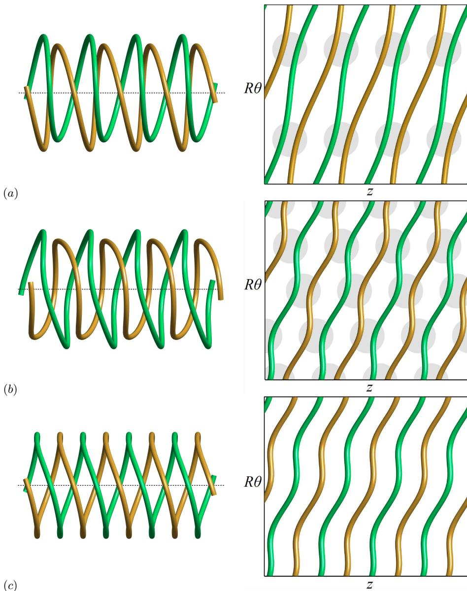
FIGURE 3. Geometrical deformation and local pairing predicted by Gupta & Loewy (1974) for the case  $h/R = 0.45$ . (a)  $k = 1$ , perturbations on both vortices are in phase at each  $z$ ; (b)  $k = 2$ , perturbations are out of phase. (c) In-phase perturbations with  $k = 2$ , no pairing occurs. Three-dimensional view on the left and developed plan view on the right. The vertical direction of the plan views is compressed by a factor 2.
