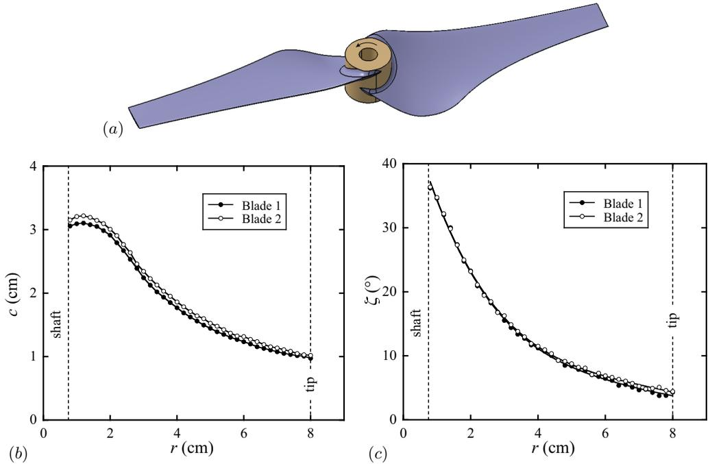
FIGURE 9. Two-bladed rotor geometry. (a) CAD drawing, and measured radial profiles of (b) chord  $c$ , and (c) twist angle  $\zeta$  of the blades.
