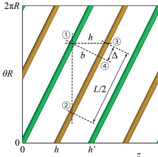
FIGURE 6. Schematic of the developed plan view of the double helix, with the definitions of the parameters employed in the analysis.
