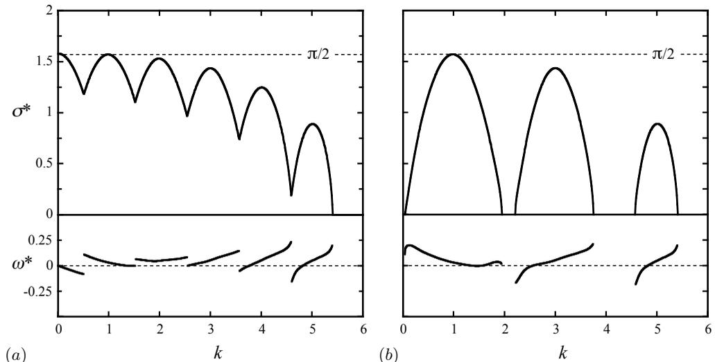
FIGURE 2. Theoretical growth rate ( $\sigma^*$ ) and frequency ( $\omega^*$ ) of the long-wave instability of two helical Rankine vortices with  $h/R = 0.41$  and  $a_e/R = 0.05$ , as predicted by Gupta & Loewy (1974). (a) Without fixed phase correlation between the two vortices; (b) for perturbations having the same phase at each  $z$  ( $\varphi = 0$ ). Frequencies are shown only for unstable modes with the highest growth rate.
