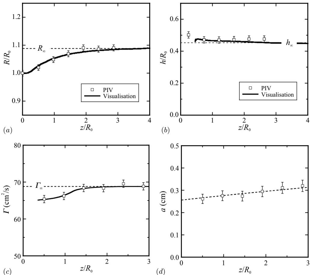
FIGURE 14. Characteristic parameters of the double-helix configuration and their downstream evolution. Geometric parameters: (a) helix radius  $R$  and (b) separation  $h$  between neighbouring helix loops. Vortex parameters: (c) circulation  $\Gamma$  and (d) core size  $a$ . The dashed line in (d) is a fit to the viscous expansion of a two-dimensional Gaussian vortex core,  $a = \sqrt{4\nu(t - t_0)}$ .
