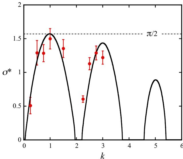
FIGURE 19. Growth rate of the long-wave instability due to local pairing, as function of wavenumber. The symbols correspond to experimental measurements, and the solid line is the theoretical prediction by Gupta & Loewy (1974) for in-phase perturbations on the two vortices. The theoretical results are obtained using the base flow parameters in table 1.
