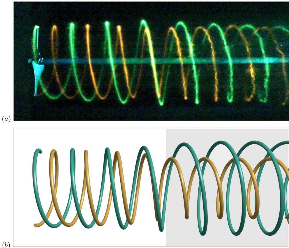
FIGURE 20. Rotor wake perturbed with a global pairing mode ( $k = 0$ ). (a) Experimental dye visualisation for the case with tip speed ratio  $\lambda = 5.4$  and radial rotor offset  $\delta/R_0 = 0.015$ ; (b) corresponding theoretical prediction (the perturbation amplitude is kept constant in the grey region).
