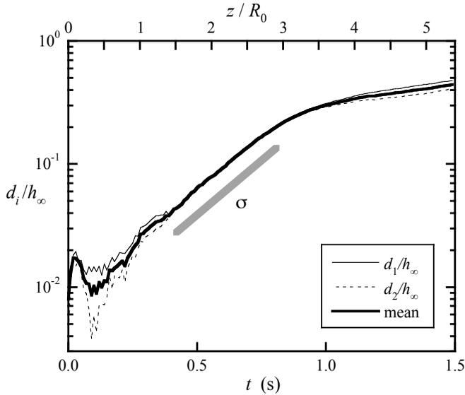
FIGURE 18. Averaged temporal evolution of the displacement amplitudes  $d_i$  ( $i = 1, 2$ ), defined in figure 17(b), for a perturbation with  $k = 1$  and  $d/h_\infty = 0.03$ . The slope of the thick grey line gives the growth rate  $\sigma$ .
