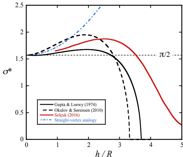
FIGURE 5. Maximum growth rate for global pairing ( $k = 0$ ), as function of the relative vortex separation  $h/R$ ; comparison of various theoretical results. The analytical studies of Gupta & Loewy (1974) and Okulov & Sørensen (2010) consider helical Rankine vortices, whereas Selçuk (2016) determines the stability of helical Lamb–Oseen vortices numerically. The equivalent core size is  $a_e/R = 0.12$  for all cases. The straight-vortex analogy corresponds to (2.7).
