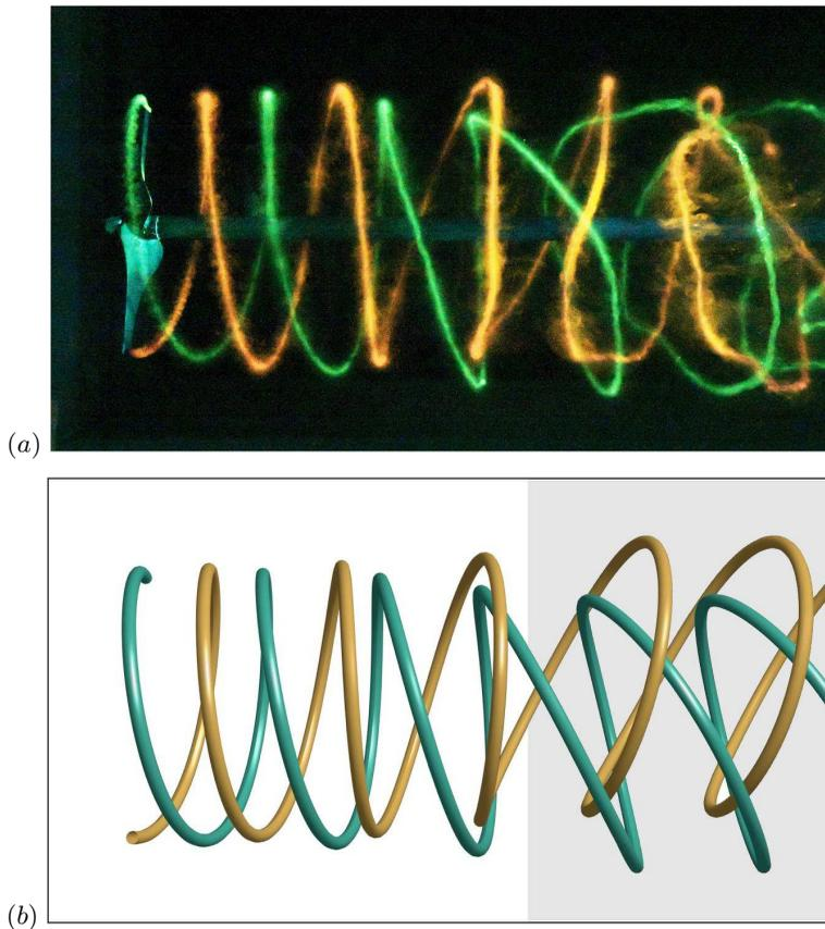
FIGURE 16. Rotor wake perturbed with a local pairing mode ( $k = 1$ ). (a) Experimental dye visualisation for  $d/h_\infty = 0.05$ ; (b) corresponding theoretical prediction (the perturbation amplitude is kept constant in the grey region).
