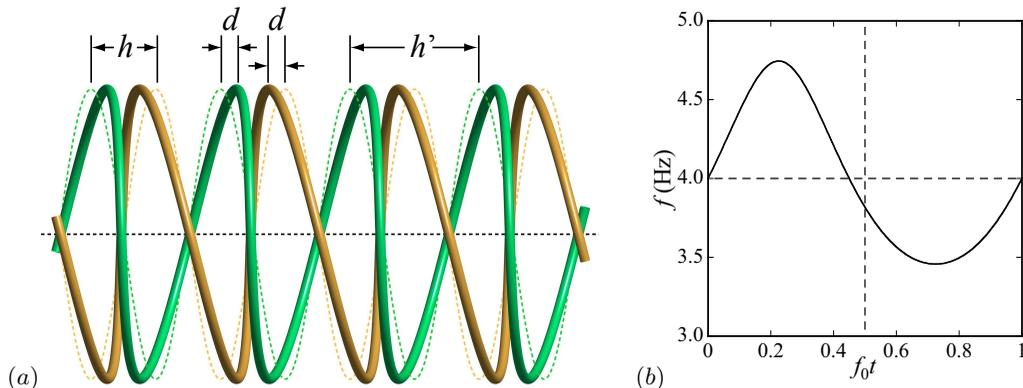
FIGURE 10. (a) Schematic of the experimental perturbation of the double helix for local pairing, consisting of an axial displacement ( $k = 1$ ,  $d/h = 0.25$ ). The dashed lines represent the unperturbed geometry. With a rigid rotor, only in-phase perturbations can be produced. (b) Modulation of the rotor rotation rate  $f$  as function of time  $t$ , for a perturbation with  $k = 1$  and  $d/h = 0.05$ .
