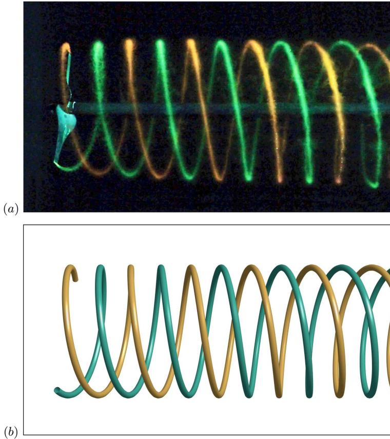
FIGURE 12. (a) Dye visualisation of the unperturbed system of two interlaced helical vortices. The rotor (radius  $R_0 = 80$  mm) is on the left, flow is from left to right. (b) Schematic of the theoretical unperturbed base flow (uniform helices), shown in a perspective projection corresponding to the experimental observation conditions (camera located at 75 cm from the rotor shaft).
