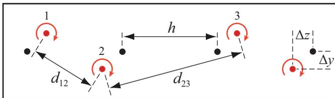
FIGURE 21. Schematic illustrating the displacement of the perturbed vortex cores in the upper half of the centre plane. The distances  $d_{12}$  and  $d_{23}$  are used to estimate the growth rate of the perturbation. The unperturbed and perturbed vortex positions are marked with black and coloured bullets, respectively.
