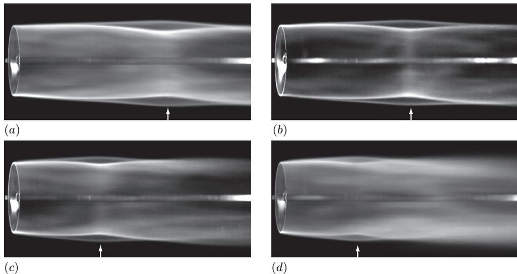
FIGURE 24. Dye patterns averaged over 22 rotor revolutions, for various tip speed ratios and  $\delta/R_0 = 0.015$ . (a)  $\lambda = 4.47$ , (b)  $\lambda = 5.40$ , (c)  $\lambda = 6.70$ , (d)  $\lambda = 8.04$ . The white arrows indicate the positions of the leapfrogging.
