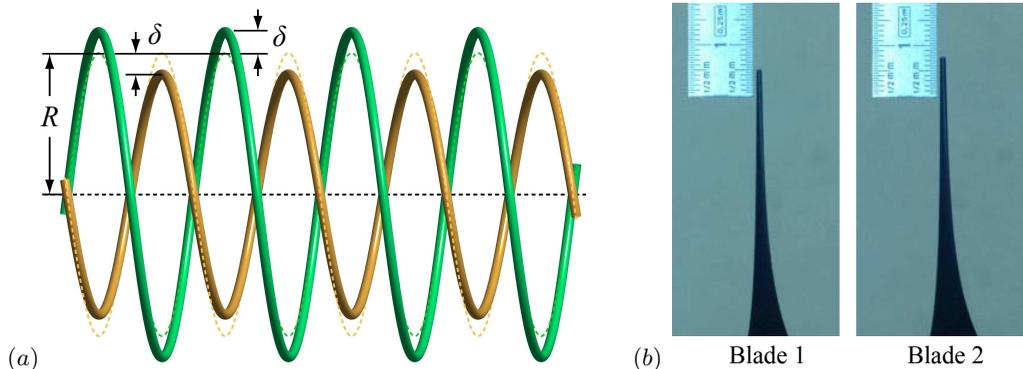
FIGURE 11. (a) Schematic of a perturbed helix configuration with  $k = 0$  (global pairing). Two helices of slightly different radius are generated by a radial offset of the two-bladed rotor. The dashed lines indicate the unperturbed geometry. (b) Photos of the blade tips used to measure the offset.
