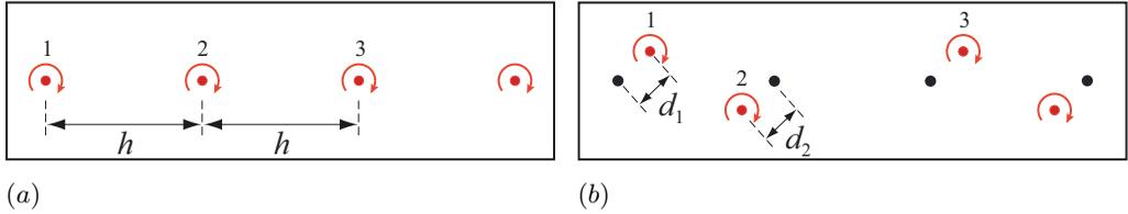
FIGURE 17. Schematic illustrating the displacement of the vortex cores in the upper half of the centre plane due to local pairing. The distances  $d_1$  and  $d_2$  are used to estimate the growth rate of the perturbation. (a) Unperturbed and (b) perturbed configuration.
