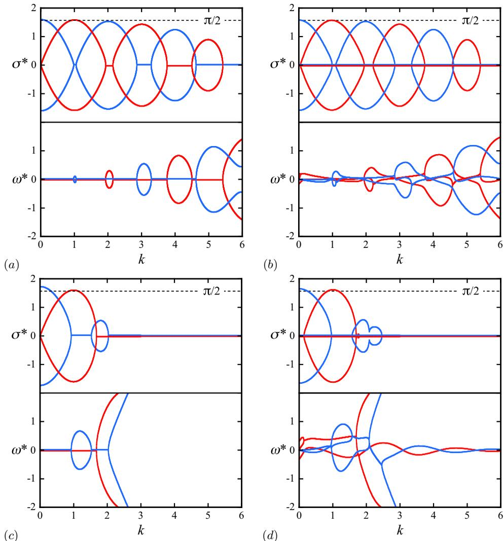
FIGURE 7. Predictions of the growth rate and frequency spectrum. Left (*a, c*): based on the results for three-dimensional pairing of straight vortices by Robinson & Saffman (1982); right (*b, d*): from the full stability analysis of the double-helix system (Gupta & Loewy 1974). Top (*a, b*):  $h/R = 0.41$  (experimental case); bottom (*c, d*):  $h/R = 1$ . In-phase (red) and out-of-phase (blue) perturbations of the two vortices,  $a_e/R = 0.05$ .
