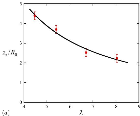
FIGURE 25. Leapfrogging distance  $z_s$  of neighbouring helix loops, as function of the tip speed ratio  $\lambda$ . The solid line is a least-squares fit of equation (6.1).
