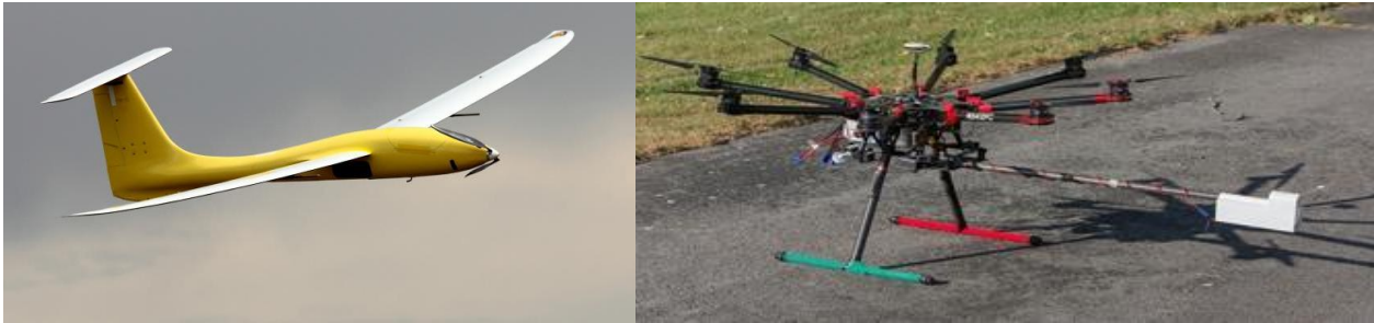
Figure 1: Example of a fixed-wing aircraft (University of Colorado, UASUSA Tempest, left) and a rotary-wing aircraft (NOAA, DJI S-1000, right).
