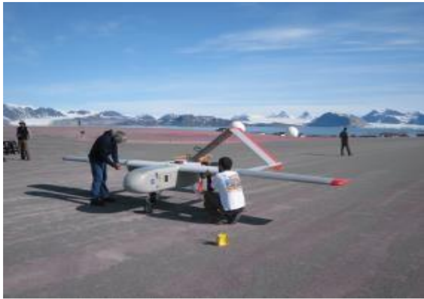
SIERRA UAS during Characterization of Arctic Sea Ice Experiment (CASIE) with LIDAR and C-band SAR (NASA, 2009)
