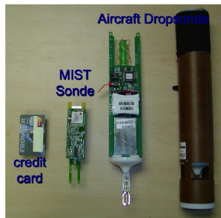
Figure 5. Size comparison of the NCAR dropsonde and driftsonde systems (Hock and Franklin, 1999).
