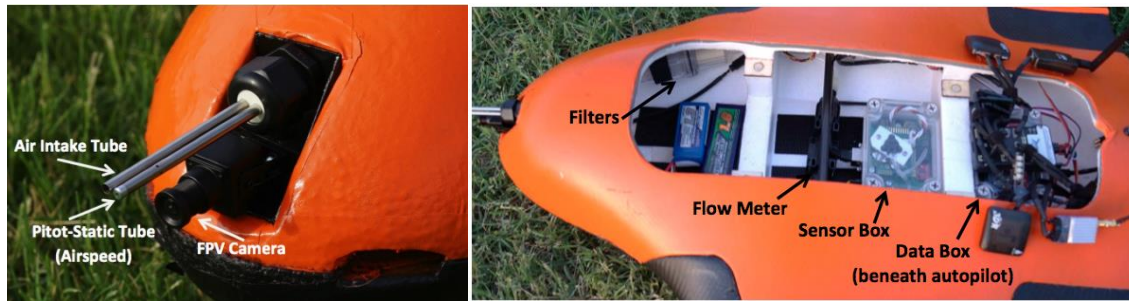
Figure 9. Sample gas sensing system with integrated environmental sensors including CO 2 & CH 4 .
