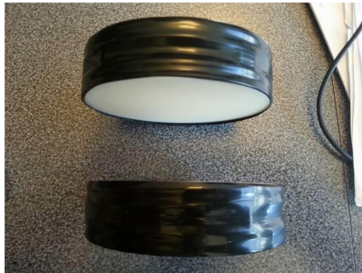
Figure 7 : Joint made of rubber and scotch tape
