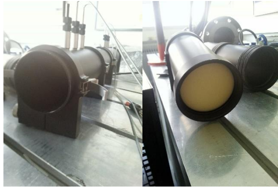
Figure 4 : Impedance tube (B&K)
