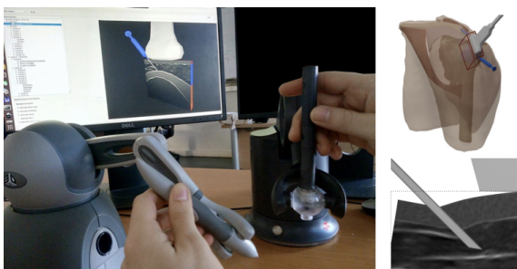
Figure 13: Our simulator which couples a graphical rendering with two haptic devices simulating probe and needle. (up) 3D models (shoulder-probe-needle); (down) zoom on tissue deformation with ultrasound view.
