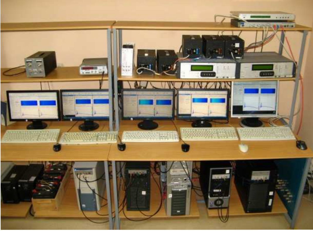
Fig. 5. The set of five DSPZ (one per telescope beam) installed in the UTR-2 receivers room.
