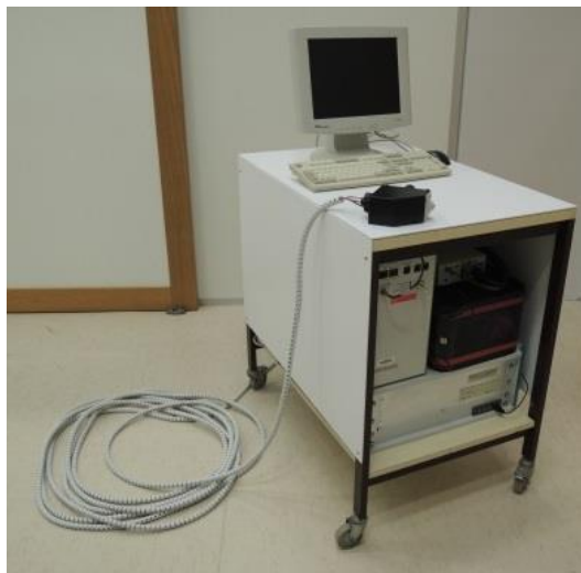
Figure 1: LIBS prototype dedicated to nuclear facilities dismantling
