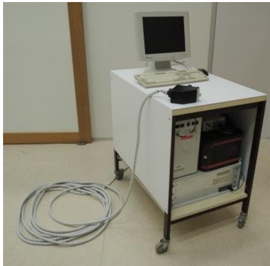
Figure 1: LIBS prototype dedicated to nuclear facilities dismantling
