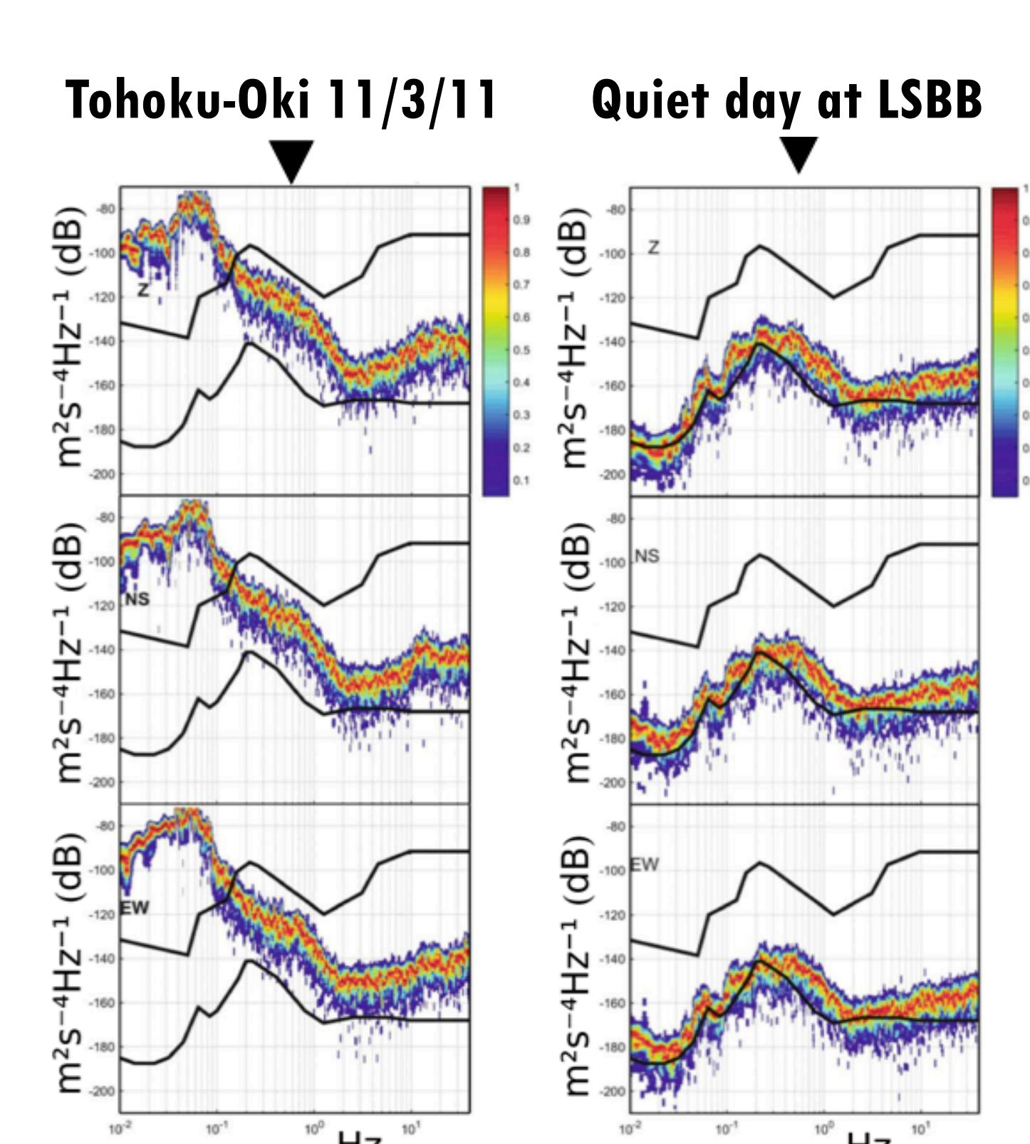
PSD (top to bottom: Z, NS, EW) vs Peterson's high and low noise models
