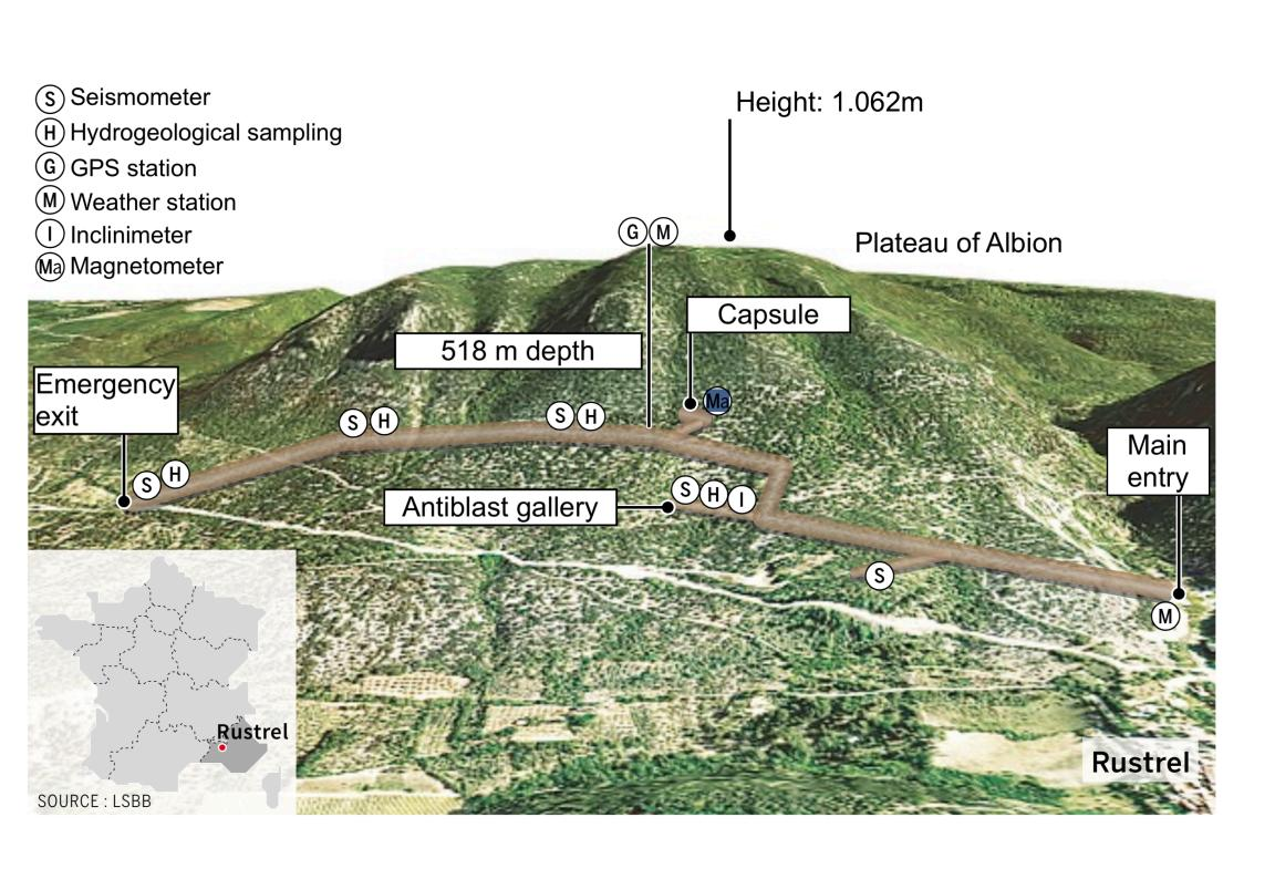
The LSBB counts with 54ha of surface and 4 km of underground galleries with depths ranging from 0 to 518 m
