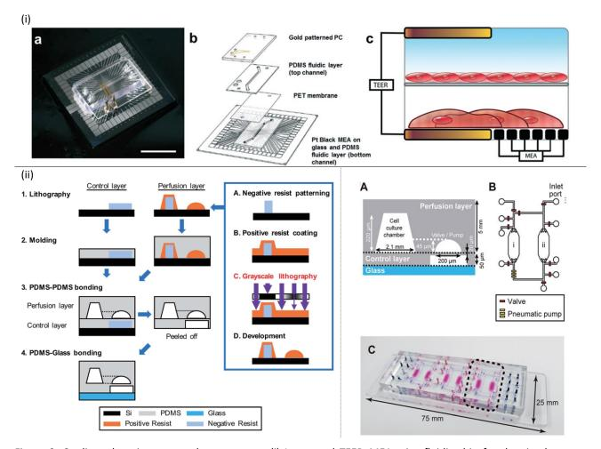
Figure 9. Cardiac-other tissues co-culture systems: (i) <u>Integrated</u> TEER–MEA <u>microfluidic</u> chip <u>for the simultaneous</u> <u>recording of cellular electrical activity and tissue barrier function</u>, reprinted <u>with permission</u> from [176]. (ii) Integrated Heart/Cancer on a Chip: left-fabrication scheme, right-microfluidic device, reprinted with permission from [178].
