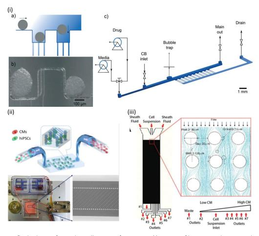
Figure 10. Microfluidic devices for cardiac cells capture/separation: (i) capture of hiPSC-CMs clusters on chip which was used for drug testing, reprinted with permission from [179]. (ii) hiPSC-CMs purification on chip via capturing the undifferentiated cells, reprinted from [180]. (iii) CMs sorting from rest cardiac cells of a neonatal rat heart based on deterministic lateral displacement, reprinted with permission from [181].
