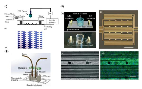
Figure 6. <u>Main</u> electrical stimulation heart-on-chip systems: (i) Dielectrophoresis and electro-orientation on chip, reprinted with permission from [153]. (ii) hiPSC-CM tissue growth on a <u>combined MEA-IDE chip.</u> Scale bar: a. 1 cm, b.1 mm, c. d. is 100  $\mu$ m. Blue: nuclei, green: cardiomyocyte troponin-T, reprinted with permission from [157]. (iii) Micromolded gelatin on <u>a commercial MEA chip</u>, reprinted with permission from [158].
