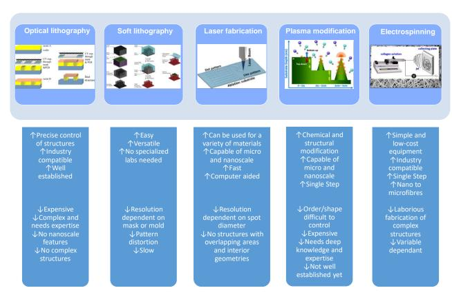
Figure 3. Basic micro and nanoengineering methods used in cardiac tissue engineering. Schematic representations of the method, followed by advantages and disadvantages for their use in cardiac tissue engineering. Figures (reprinted with permission) are modified from the following: optical lithography from [21], soft lithography from [34], laser ablation from [64], plasma modification from [114], and electrospinning from [90].
