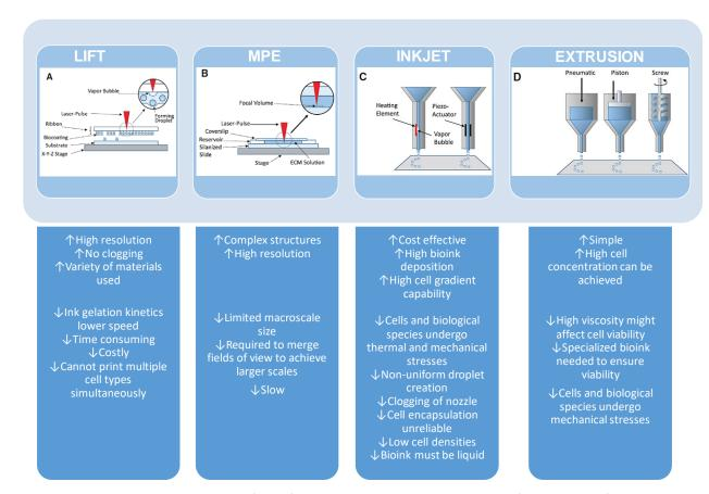
Figure 5. Schematic representations of the four most widely used techniques of 3D printing for cardiac tissue engineering (reprinted and modified from [121]). (A) Laser-assisted bioprinting (LAB) which is based on laser-induced forward transfer (LIFT). (B) Multiphoton excitation (MPE) which is also called stereolithography. (C) Inkjet printing. (D) Microextrusion ink deposition. The basic advantages and disadvantages for each method for 3D bioprinting are cited below each schematic.
