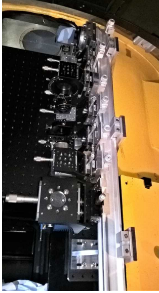
Figure 1. Shack-Hartmann wavefront sensor installed at THEMIS telescope.
