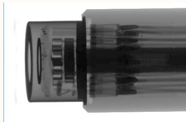
Tomography scan of X-PIPS detector
