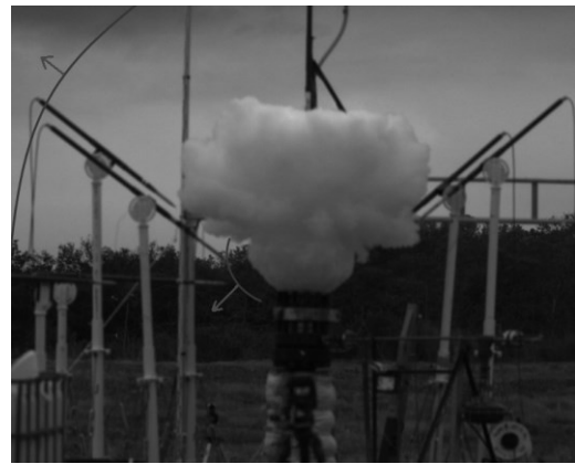
Figure 9. High speed camera capture of the blast waves
