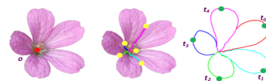
Fig. 10: Petal contour detection technique proposed in [40]. (Left image) Initially, the center of the flower is located by user assistance (red dot). (Middle image) The intersection points of the petals are located as yellow dots. (Right image) The petals tips are located as the green dots.
