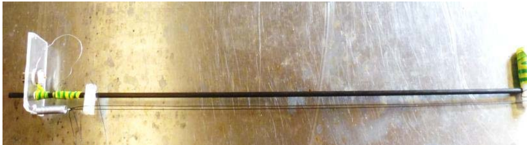
Figure 3: Illustration of handmade capacitive probe for water elevation measurements
