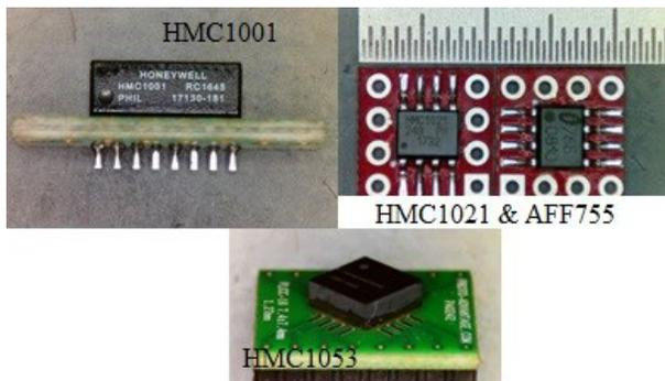
Figure 3: AMR sensors mounted on their PCB.
