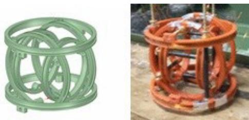
Figure 1: Helmholtz cell formed by 3 paired coils ( $\varnothing$  110 mm / 96 mm / 76 mm). Left: sketch of the ABS supports. Right: Picture of the assembled coils.
