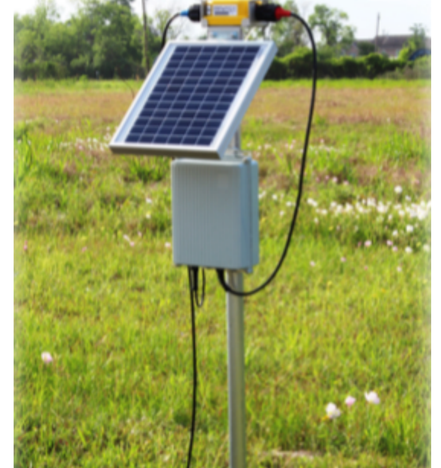
Example of autonomous Nodes, Geospace (USA)
