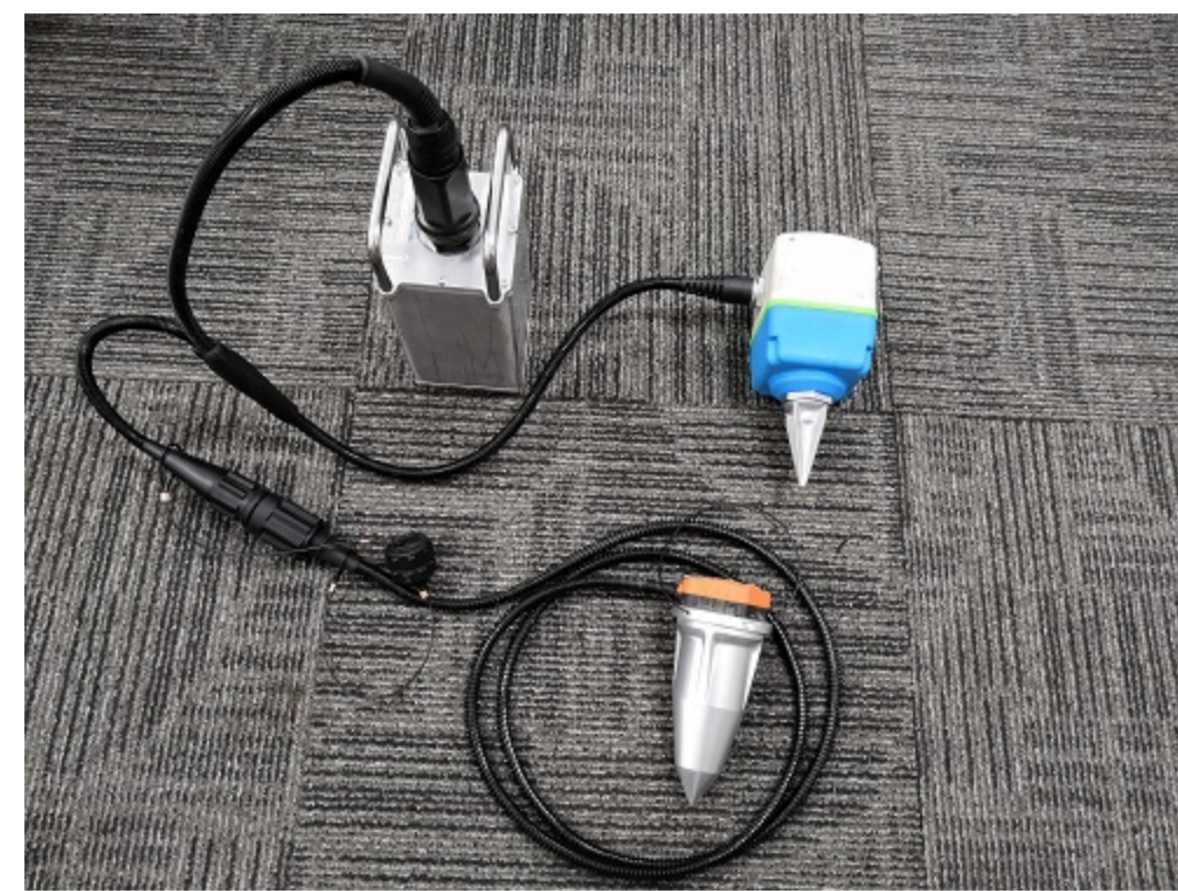
DTCC system, China Derived SmartSolo node Prototype under development
