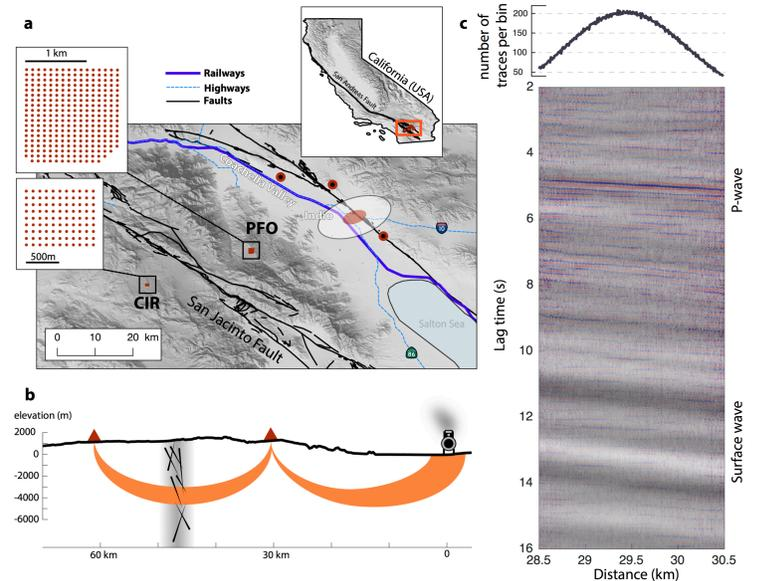
**Results of an exploratory seismic experiment in Southern California in 2017** (Brenguier F. et al, (2019). Train traffic as a powerful noise source for monitoring active Faults with seismic interferometry, [10.1029/2019GL083438](https://doi.org/10.1029/2019GL083438))
