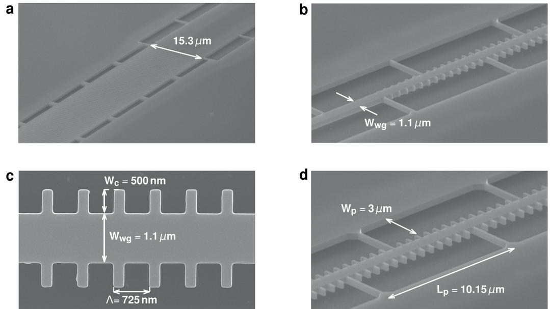
**Figure 3.** Scanning electron microscope (SEM) image of the fabricated silicon membrane Bragg filter (a) fiber-chip grating coupler, (b) transition between strip waveguide and grating, (c) detail of the filter geometry and (d) side view showing anchoring pillars.
