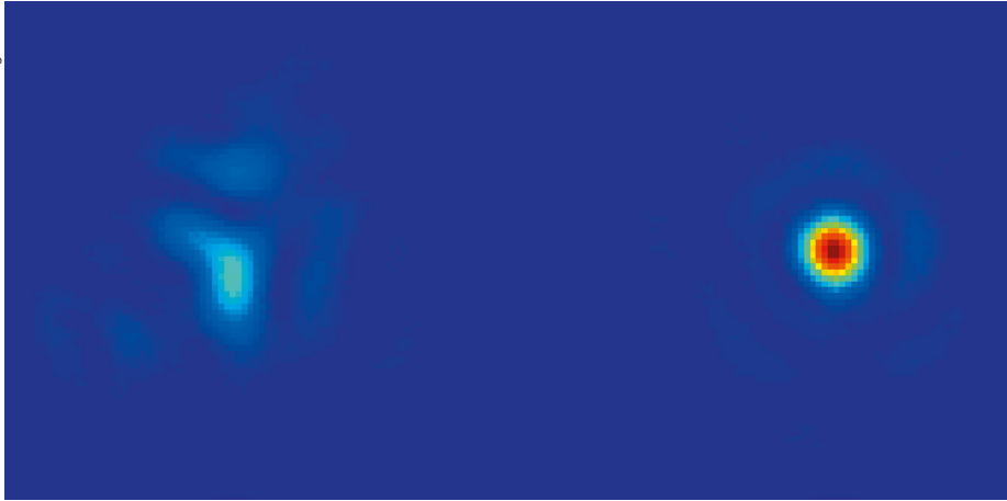
Figure 6. Acquisition of a star with the infrared Strehl camera ( H -band) in open loop (left) and in closed loop (right) for quasi-instantaneous Strehl measurement (50 ms integration time) during the stand-alone verification of AT1.
