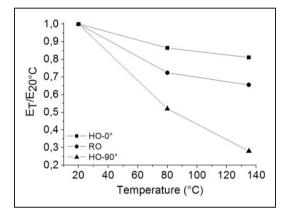
Figure 6. Evolutions of the relative Young's modulus of HO-0°, RO, and HO-90° samples at different temperatures.
