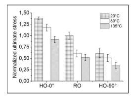
**Figure 5.** Normalized ultimate stress of oriented and nonoriented samples at 20°C, 80°C, and 135°C; (normalized value = current value/average ultimate stress ( $\sigma_r$ ) value obtained for tests performed at 20°C on RO-A-SMC).
