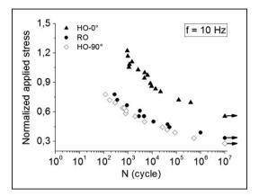
Figure 8. Normalized Wöhler curves for HO-0°, RO, and HO-90° samples at 10 Hz.
