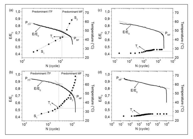
Figure 11. Evolutions of the relative Young's modulus (E/E<sub>0</sub>) and the self-heating phenomenon during fatigue tests: (a) f = 100 Hz and  $\sigma_{max} = 0.55 \sigma_{r(RO)}$ , (b) f = 100 Hz and  $\sigma_{max} = 0.40 \sigma_{r(RO)}$ , (c) f = 10 Hz and  $\sigma_{max} = 0.55 \sigma_{r(RO)}$  and (d) f = 10 Hz and  $\sigma_{max} = 0.40 \sigma_{r(RO)}$ .
