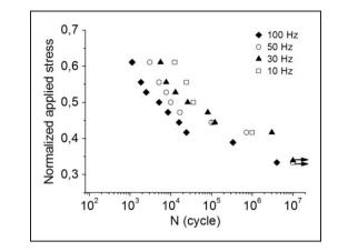
**Figure 9.** Normalized Wöhler curves at different frequencies for RO samples.
