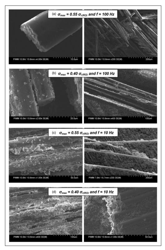
Figure 13. Fracture surface observation performed at different loading conditions: (a)  $\sigma_{max} = 0.55 \sigma_{r(RO)}$  and f = 100 Hz, (b)  $\sigma_{max} = 0.40 \sigma_{r(RO)}$  and f = 100 Hz, (c)  $\sigma_{max} = 0.55 \sigma_{r(RO)}$  and f = 10 Hz and (d)  $\sigma_{max} = 0.40 \sigma_{r(RO)}$  and f = 10 Hz.
