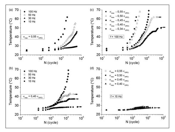
**Figure 10.** Temperature variation at different frequencies and amplitudes for RO samples: (a)  $\sigma_{max} = 0.55 \sigma_{r(RO)}$  and different frequencies, (b)  $\sigma_{max} = 0.40 \sigma_{r(RO)}$  ultimate stress and different frequencies, (c) f = 100 Hz and different amplitudes and (d) f = 10 Hz and different amplitudes.
