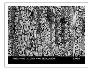
**Figure 1.** Typical microstructure of A-SMC observed by mean of a SEM: randomly oriented bundle of fibers.
