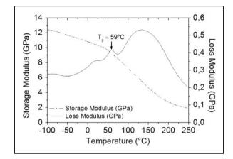
**Figure 3.** DMTA scan showing the types of transitions for RO-A-SMC sample.
