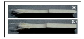
Figure 7. Macroscopic failure appearance of HO-90° sample loaded at (a)  $20^{\circ}$ C and (b)  $135^{\circ}$ C.
