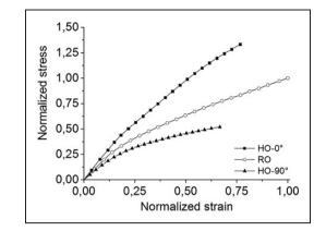
**Figure 4.** Normalized quasi-static tensile behavior of A-SMC composite at room temperature. One can mention that normalized stress (respectively strain) = stress (respectively strain)/ultimate stress (respectively strain) obtained for tests performed on RO-A-SMC serving as a reference.
