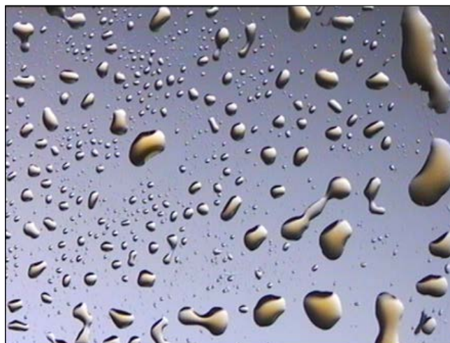
Figure 3: A typical residue on the MgF 2 window under the microscope (x60, white light). Droplets of organic molecular oily residue are observed. They represent a total mass of soluble matter around 100 µg. The yellow color is always observed on these materials, nicknamed “yellow stuff” around 1980 by J. Mayo Greenberg. Picture size is around 1x1 mm 2 (Modica, 2014).
