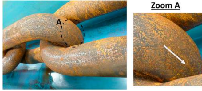
Fig. 16. Fatigue crack at the Crown.
