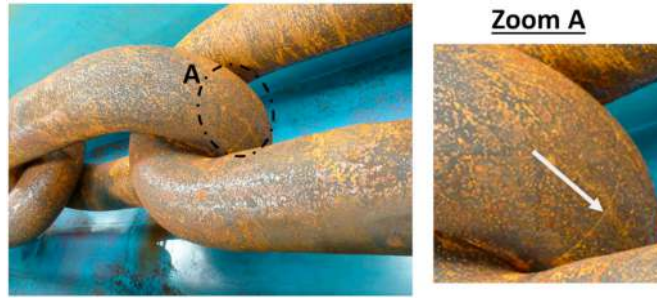
Fig. 16. Fatigue crack at the Crown.
