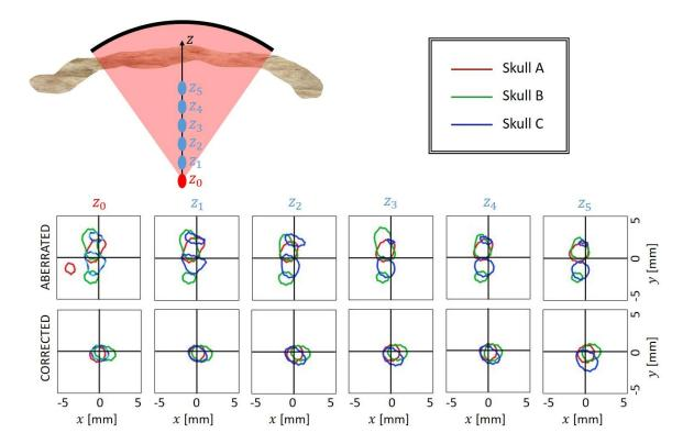
for every steering position along the z axis. Compared to the reference (steering-less position at  $x_0$ ), the acoustic intensity decreases by 37% experimentally (and by 60% numerically) for a 10mm steering along the z axis. The -3dB surface does not significantly increase with steering; it varies from 2.94mm<sup>2</sup> (no steering) to 3.72mm<sup>2</sup> (10mm steering) in the experimental case, and from 1.97mm<sup>2</sup> to 2.77m<sup>2</sup> in the numerical case.
