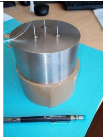
Fig.10b : Mock-up for feedthrough welding qualification
